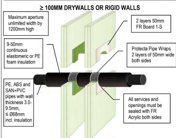
**INSULATED PE PIPES FIRE RESISTANCE EI 60 C/C (E 60)**
